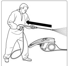
Bear in mind that during cleaning tasks with a high-pressure water jet a significant recoil at the lance arises. Please stand firmly. (see technical data on page 4).
