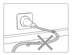
Only use power cables which are in perfect working order! Do not damage the power cable or repair it incorrectly!
