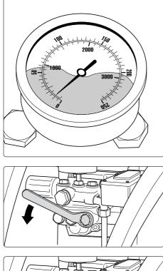
The pressure gauge shows little pressure despite fully turned up pressure regulation. The water from the lance comes in squirts. The HP hose vibrates.
