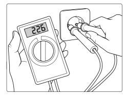
If there are too many collectors in your proximity connected to the network at the same time, the available voltage and the current intensity may decline. Consequently the motor of the high-pressure cleaner does not start or even blows.
