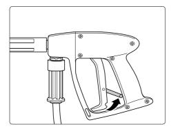
Apply the safety catch on the spray gun after each use, in order to prevent unintentional spraying!
