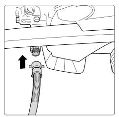
Attach suction hose. The inner diameter of the hose must be at least  $1/2^{\circ}$  = 12.7 mm.
