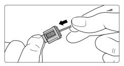
Take out valve body (with green or red plastic coating) and O-ring by means of needle nose pliers. Check O-ring for damage. In case of a damage the O-ring has to be replaced.
