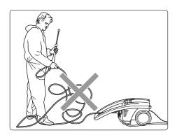
Never pull the high pressure hose if it has formed kinks or "nooses"! Never pull the hose over sharp edges!
