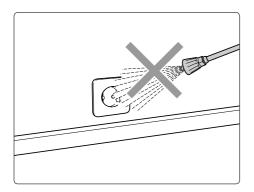
Never direct the water jet at a power socket!
